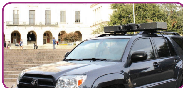
FIG 5 The University of Texas’ Sensorium is a platform for automated and connected vehicle perception research. It includes stereo visible-light cameras, an industrial-grade IMU, an automotive radar unit, a dual-antenna, a dual-frequency software-defined GNSS receiver, 4G cellular connectivity, and a powerful internal computer.
