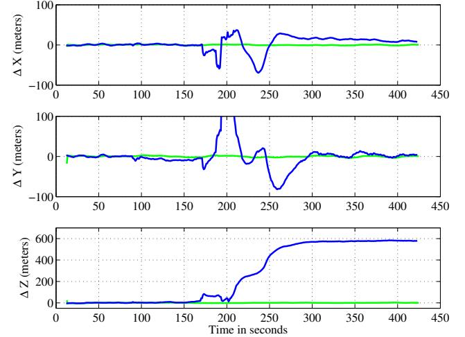
Fig. 20. Scenario 4: Time history of receiver ECEF position deviation from mean. In each panel, the green trace shows the receiver's unspoofed response and the blue trace shows the receiver's spoofed response.
