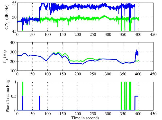
Fig. 24. Scenario 5: Time history of  $C/N_0$  (top panel),  $f_D$  (center panel), and the phase trauma indicator (bottom panel) corresponding to a single signal being spoofed. In each panel, the green trace shows the receiver's unspoofed response and the blue trace shows the receiver's spoofed response. The unspoofed and spoofed phase trauma indicators have different amplitudes only for visual clarity.
