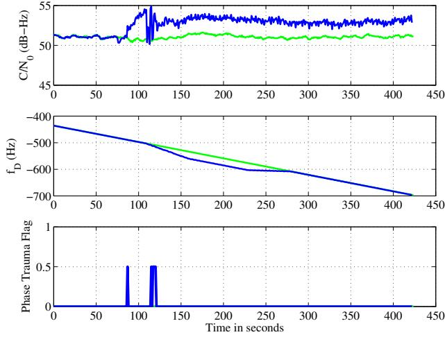
Fig. 9. Scenario 2: Time history of  $C/N_0$  (top panel),  $f_D$  (center panel), and the phase trauma indicator (bottom panel) corresponding to a single signal being spoofed. In each panel, the green trace shows the receiver's unspoofed response and the blue trace shows the receiver's spoofed response.
