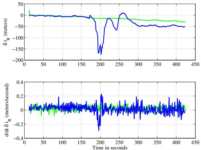
Fig. 21. Scenario 4: Time history of  $\delta t_R$  (top panel) and  $d/dt \delta t_R$  (bottom panel). In each panel, the green trace shows the receiver's unspoofed response and the blue trace shows the receiver's spoofed response.
