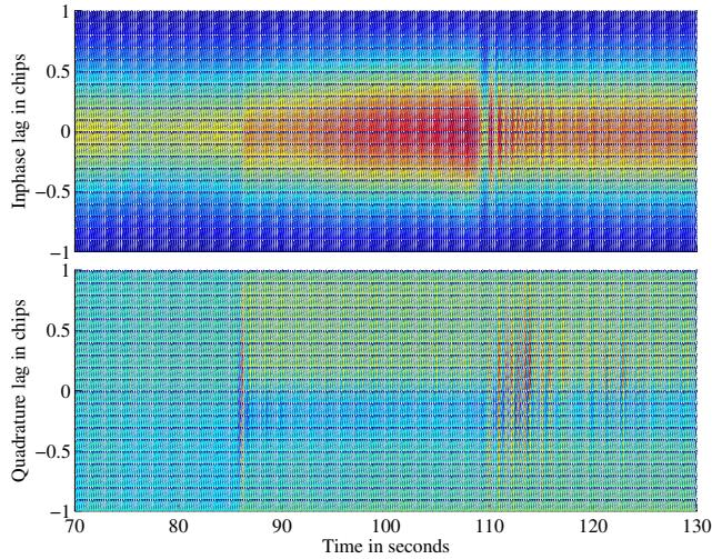
Fig. 12. Scenario 2: Navigation-data-free output time history of 21 complex correlation taps uniformly spaced at an interval of 0.1 C/A code chips and centered at the receiver's prompt tap. In-phase (top panel) and quadrature (bottom panel) accumulations are based on 2-second coherent summations.
