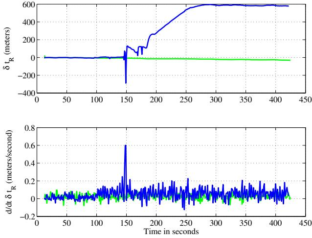
Fig. 16. Scenario 3: Time history of  $\delta t_R$  (top panel) and  $d/dt \delta t_R$  (bottom panel). In each panel, the green trace shows the receiver's unspoofed response and the blue trace shows the receiver's spoofed response.
