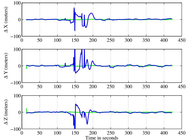
Fig. 15. Scenario 3: Time history of receiver ECEF position deviation from mean. In each panel, the green trace shows the receiver's unspoofed response and the blue trace shows the receiver's spoofed response.
