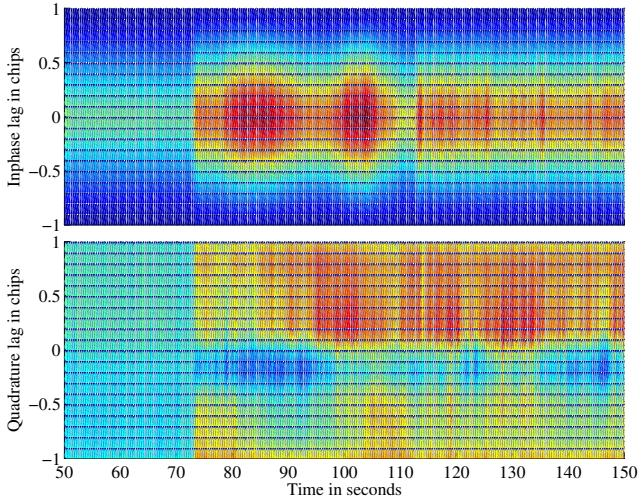
Fig. 27. Scenario 5: Navigation-data-free output time history of 21 complex correlation taps uniformly spaced at an interval of 0.1 C/A code chips and centered at the receiver's prompt tap. In-phase (top panel) and quadrature (bottom panel) accumulations are based on 4-second coherent summations.
