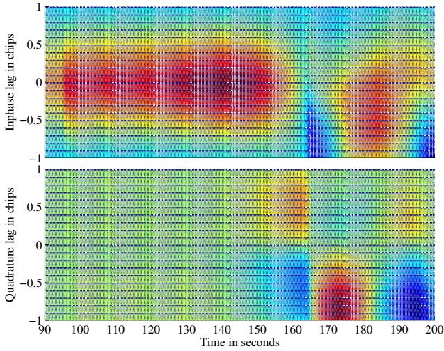
Fig. 17. Scenario 3: Navigation-data-free output time history of 21 complex correlation taps uniformly spaced at an interval of 0.1 C/A code chips and centered at the receiver's prompt tap. In-phase (top panel) and quadrature (bottom panel) accumulations are based on 4-second coherent summations.
