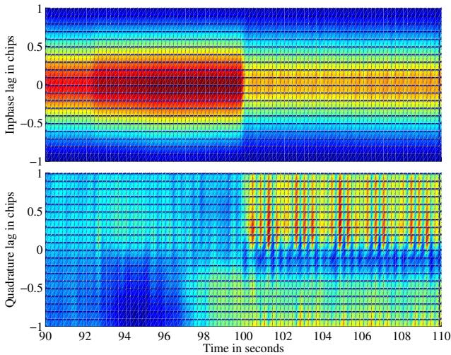
Fig. 7. Scenario 1: Navigation-data-free output time history of 21 complex correlation taps uniformly spaced at an interval of  $0.1 C/A$  code chips and centered at the receiver's prompt tap. In-phase (top panel) and quadrature (bottom panel) accumulations are based on 2-second coherent summations.
