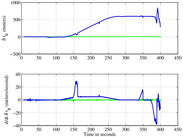
Fig. 26. Scenario 5: Time history of  $\delta t_R$  (top panel) and  $d\delta t_R/dt$  (bottom panel). In each panel, the green trace shows the receiver's unspoofed response and the blue trace shows the receiver's spoofed response.
