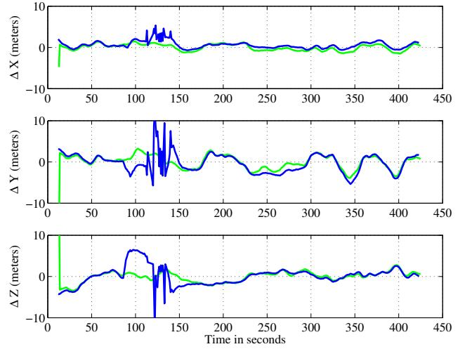
Fig. 10. Scenario 2: Time history of receiver ECEF position deviation from mean. In each panel, the green trace shows the receiver's unspoofed response and the blue trace shows the receiver's spoofed response.
