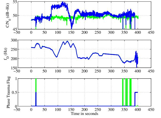
Fig. 29. Scenario 6: Time history of  $C/N_0$  (top panel),  $f_D$  (center panel), and the phase trauma indicator (bottom panel) corresponding to a single signal being spoofed. In each panel, the green trace shows the receiver's unspoofed response and the blue trace shows the receiver's spoofed response. The unspoofed and spoofed phase trauma indicators have different amplitudes only for visual clarity.
