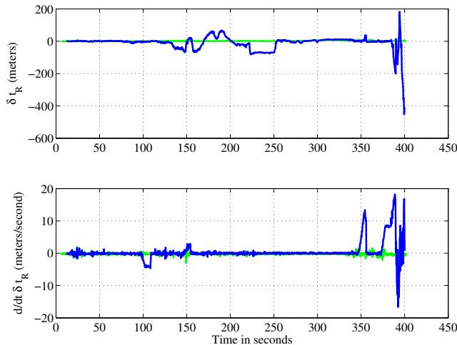
Fig. 31. Scenario 6: Time history of  $\delta t_R$  (top panel) and  $d/dt \delta t_R$  (bottom panel). In each panel, the green trace shows the receiver's unspoofed response and the blue trace shows the receiver's spoofed response.
