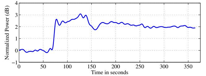
Fig. 28. Scenario 6: Time history of normalized power in a 2-MHz band centered at GPS L1.
