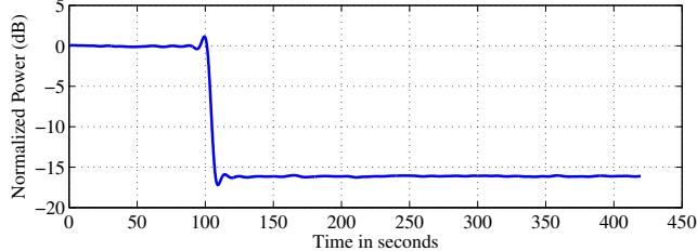
Fig. 3. Scenario 1: Time history of normalized power in a 2-MHz band centered at GPS L1.
