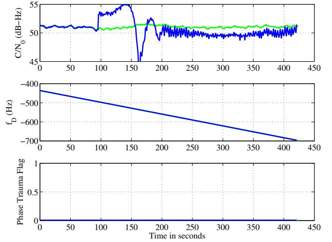
Fig. 14. Scenario 3: Time history of  $C/N_0$  (top panel),  $f_D$  (center panel), and the phase trauma indicator (bottom panel) corresponding to a single signal being spoofed. In each panel, the green trace shows the receiver's unspoofed response and the blue trace shows the receiver's spoofed response.
