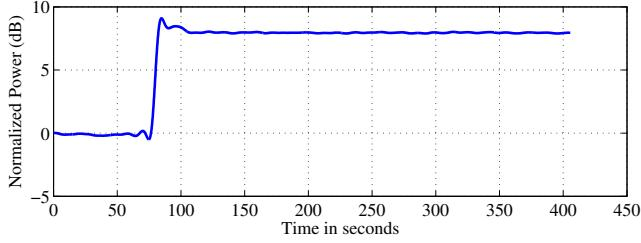
Fig. 8. Scenario 2: Time history of normalized power in a 2-MHz band centered at GPS L1.
