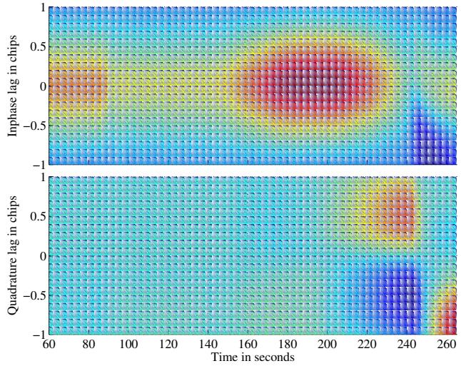
Fig. 22. Scenario 4: Navigation-data-free output time history of 21 complex correlation taps uniformly spaced at an interval of 0.1 C/A code chips and centered at the receiver's prompt tap. In-phase (top panel) and quadrature (bottom panel) accumulations are based on 4-second coherent summations.
