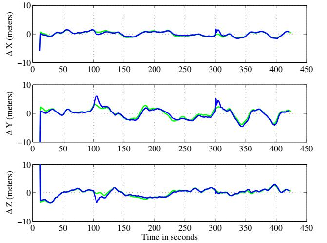
Fig. 5. Scenario 1: Time history of receiver ECEF position deviation from mean. In each panel, the green trace shows the receiver's unspoofed response and the blue trace shows the receiver's spoofed response.
