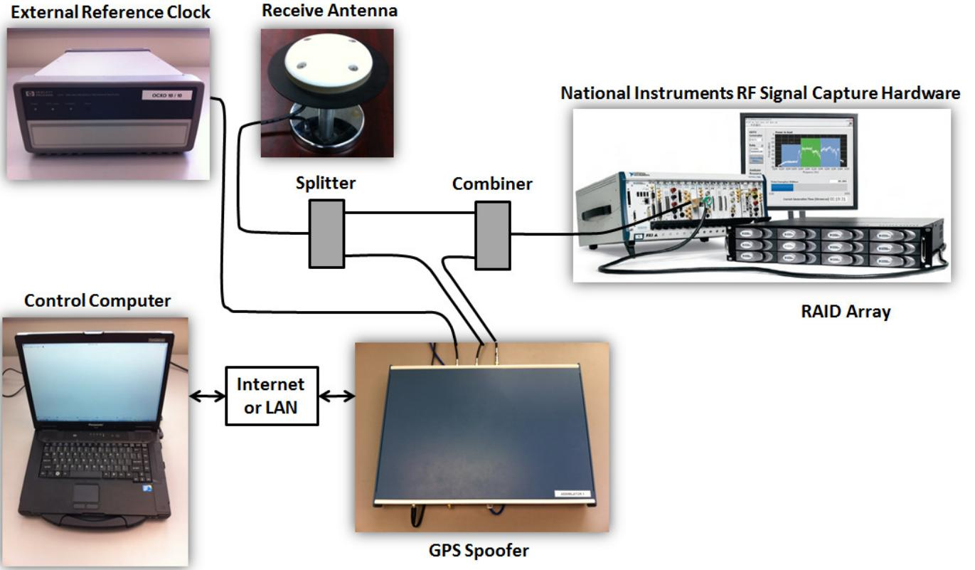
Fig. 2. Diagram of the TEXBAT recording setup.
