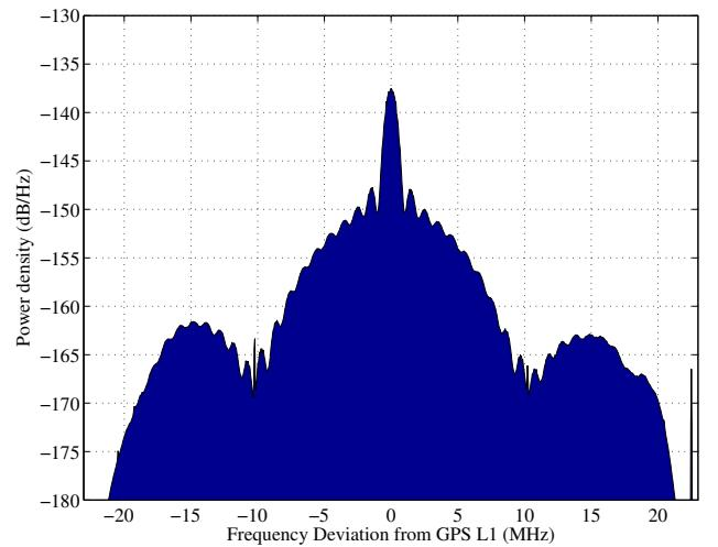
Fig. 1. Power spectral density estimate of the GPS signal corresponding to PRN 31 as received on 22 April, 2003 by the Stanford 46-meter-diameter radio telescope (original data courtesy of Dennis Akos). The complex sampling rate of the digitized data was 46.08 Msps.
