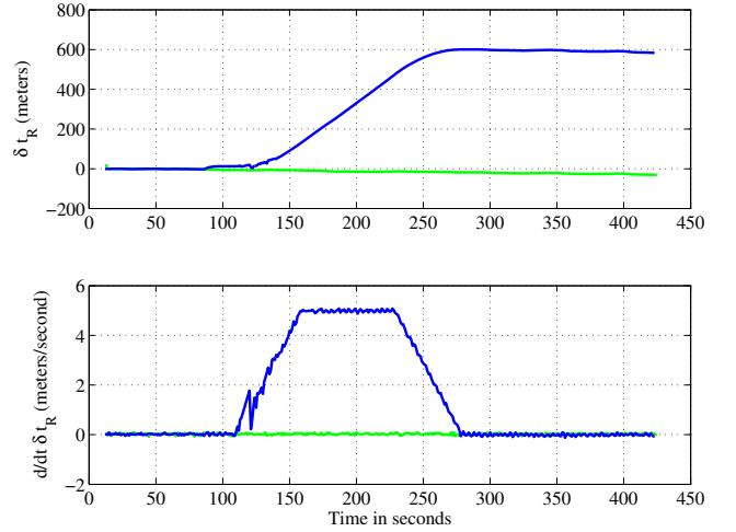
Fig. 11. Scenario 2: Time history of  $\delta t_R$  (top panel) and  $d/dt \delta t_R$  (bottom panel). In each panel, the green trace shows the receiver's unspoofed response and the blue trace shows the receiver's spoofed response.
