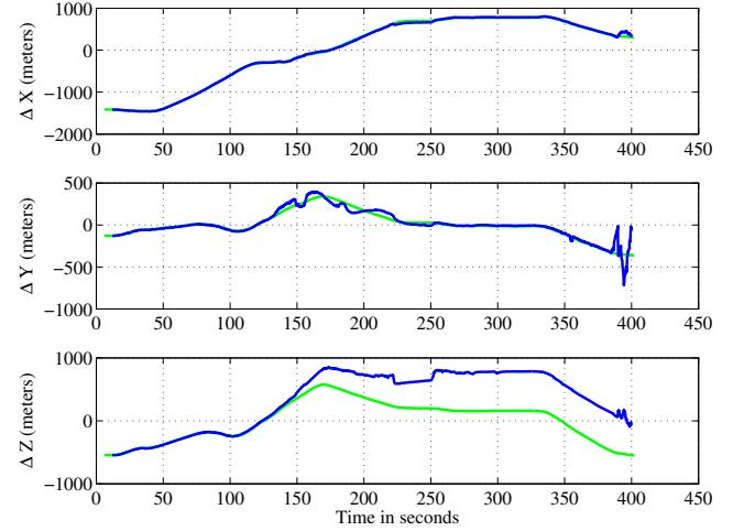
Fig. 30. Scenario 6: Time history of receiver ECEF position deviation from mean. In each panel, the green trace shows the receiver's unspoofed response and the blue trace shows the receiver's spoofed response.
