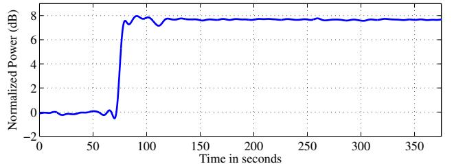
Fig. 23. Scenario 5: Time history of normalized power in a 2-MHz band centered at GPS L1.
