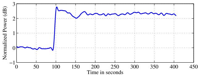
Fig. 13. Scenario 3: Time history of normalized power in a 2-MHz band centered at GPS L1.
