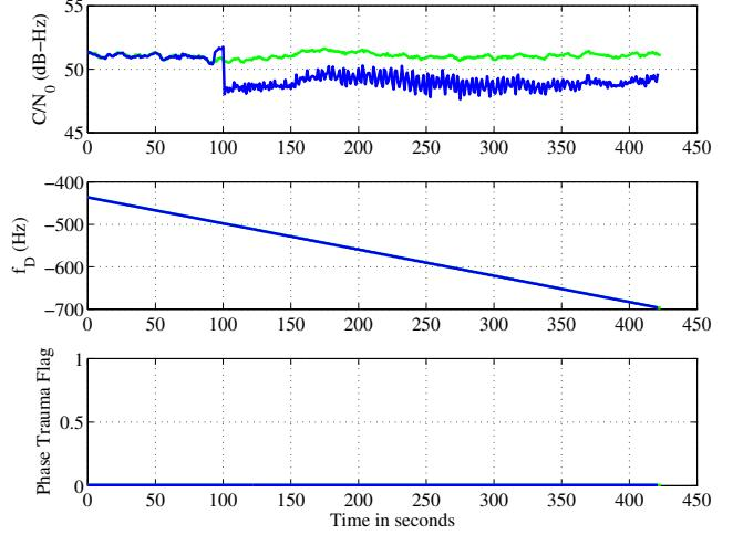
Fig. 4. Scenario 1: Time history of  $C/N_0$  (top panel),  $f_D$  (center panel), and the phase trauma indicator (bottom panel) corresponding to a single signal being spoofed. In each panel, the green trace shows the receiver's unspoofed response and the blue trace shows the receiver's spoofed response.
