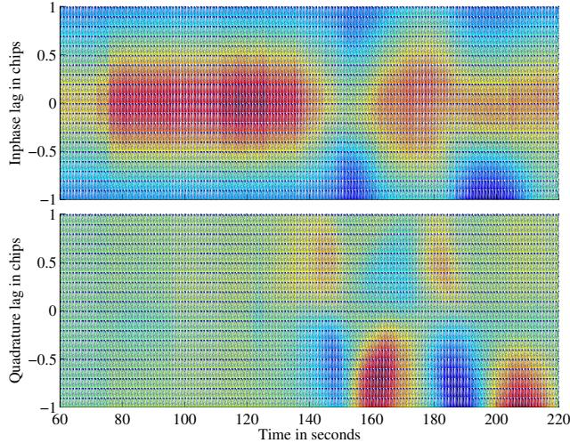
Fig. 32. Scenario 6: Navigation-data-free output time history of 21 complex correlation taps uniformly spaced at an interval of 0.1 C/A code chips and centered at the receiver's prompt tap. In-phase (top panel) and quadrature (bottom panel) accumulations are based on 4-second coherent summations.
