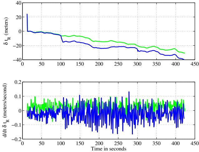
Fig. 6. Scenario 1: Time history of  $\delta t_R$  (top panel) and  $d/dt \delta t_R$  (bottom panel). In each panel, the green trace shows the receiver's unspoofed response and the blue trace shows the receiver's spoofed response.
