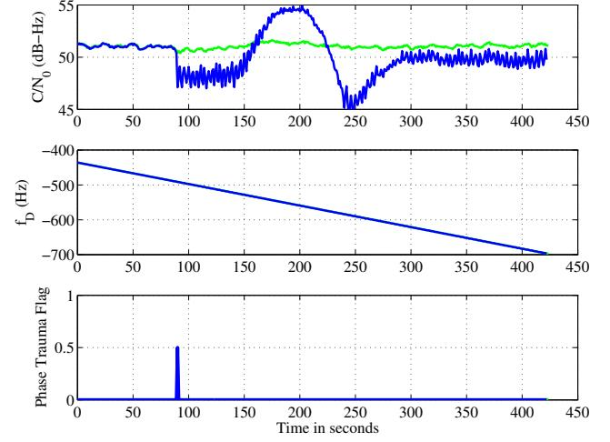
Fig. 19. Scenario 4: Time history of  $C/N_0$  (top panel),  $f_D$  (center panel), and the phase trauma indicator (bottom panel) corresponding to a single signal being spoofed. In each panel, the green trace shows the receiver's unspoofed response and the blue trace shows the receiver's spoofed response.
