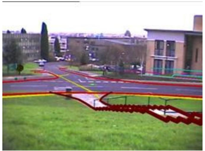
Fig. 3. An image produced by an augmented reality system developed by researchers at the University of Nottingham. This image shows subsurface utilities visualized in their correct location relative to the real world image in the background [4].
