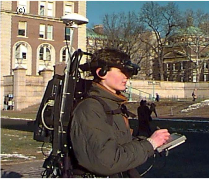
Fig. 4. An augmented reality system developed by researchers at Columbia University for providing users with information about their surroundings [5].
