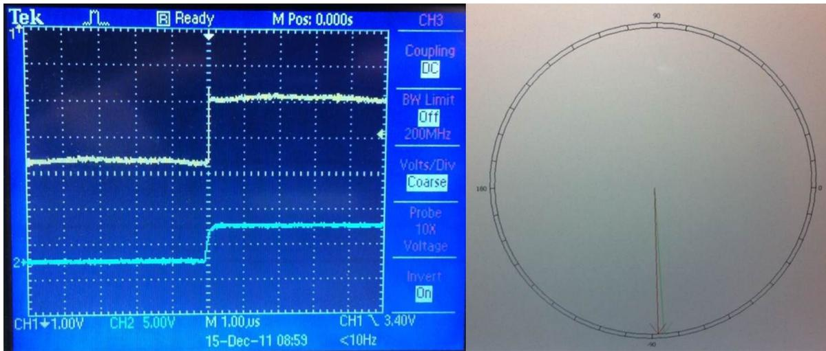
Fig. 8. Pictures of the oscilloscope (left) and synchrophasor (right) screen at the start of the test, which is marked as point 1 in Fig. 7.
