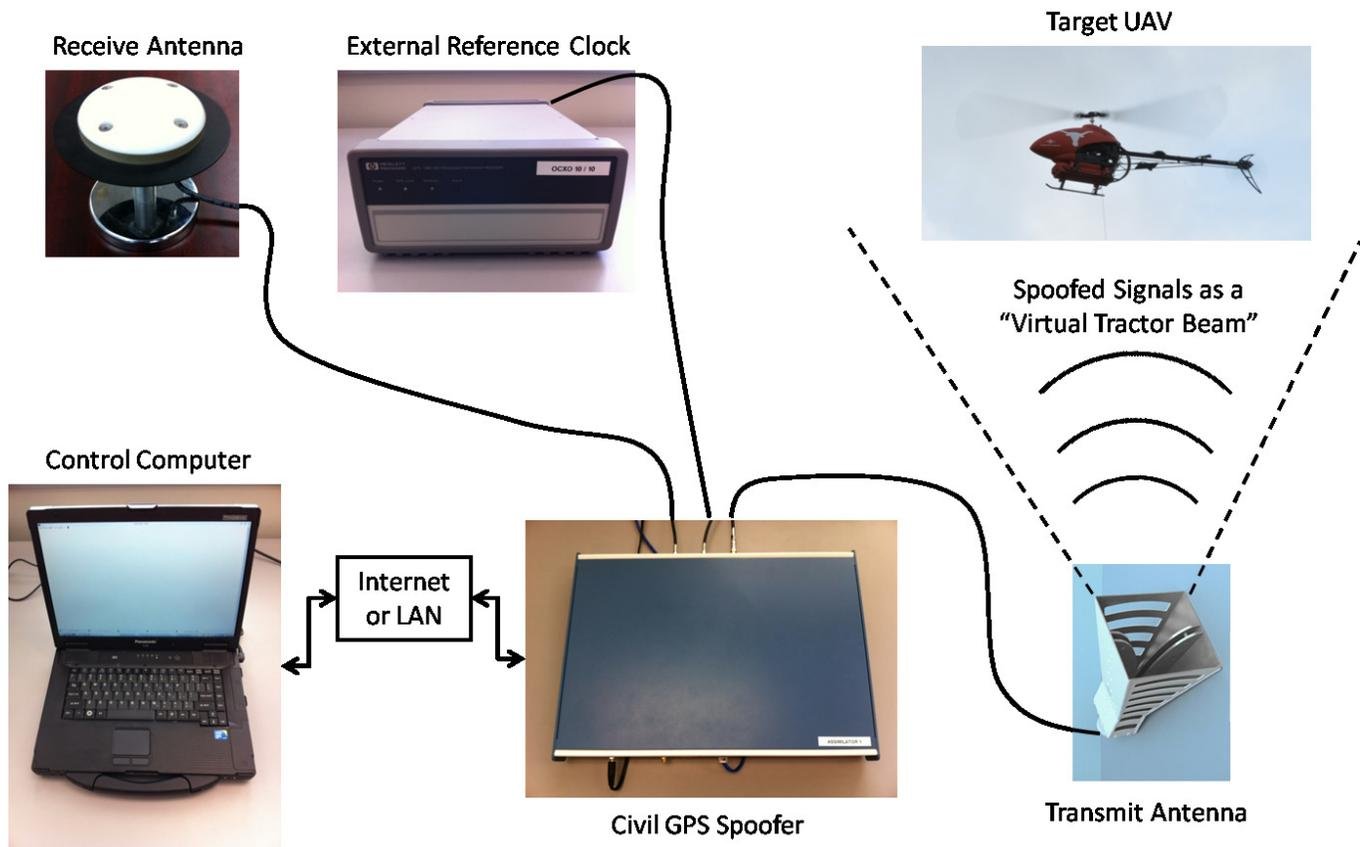
Fig. 5. A schematic of the UAV test setup.
