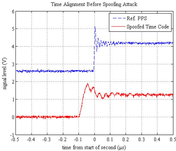
Fig. 13. Time alignment of the reference PPS (top blue dashed line) and the spoofed IRIG-B time code (bottom red line) before the spoofing attack began.
