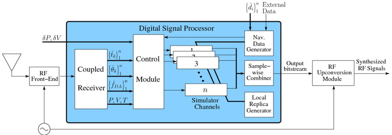
Fig. 2. A block diagram of the Spoofers.
