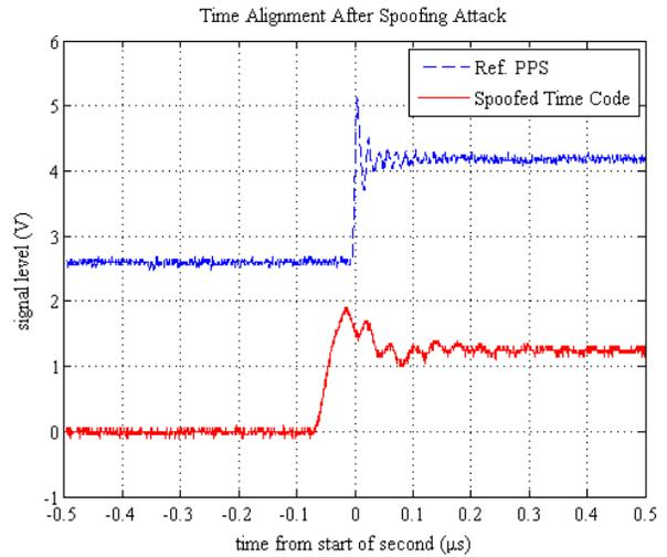
Fig. 15. Time alignment of the reference PPS (top blue dashed line) and the spoofed IRIG-B time code (bottom red line) after the spoofing attack ended.
