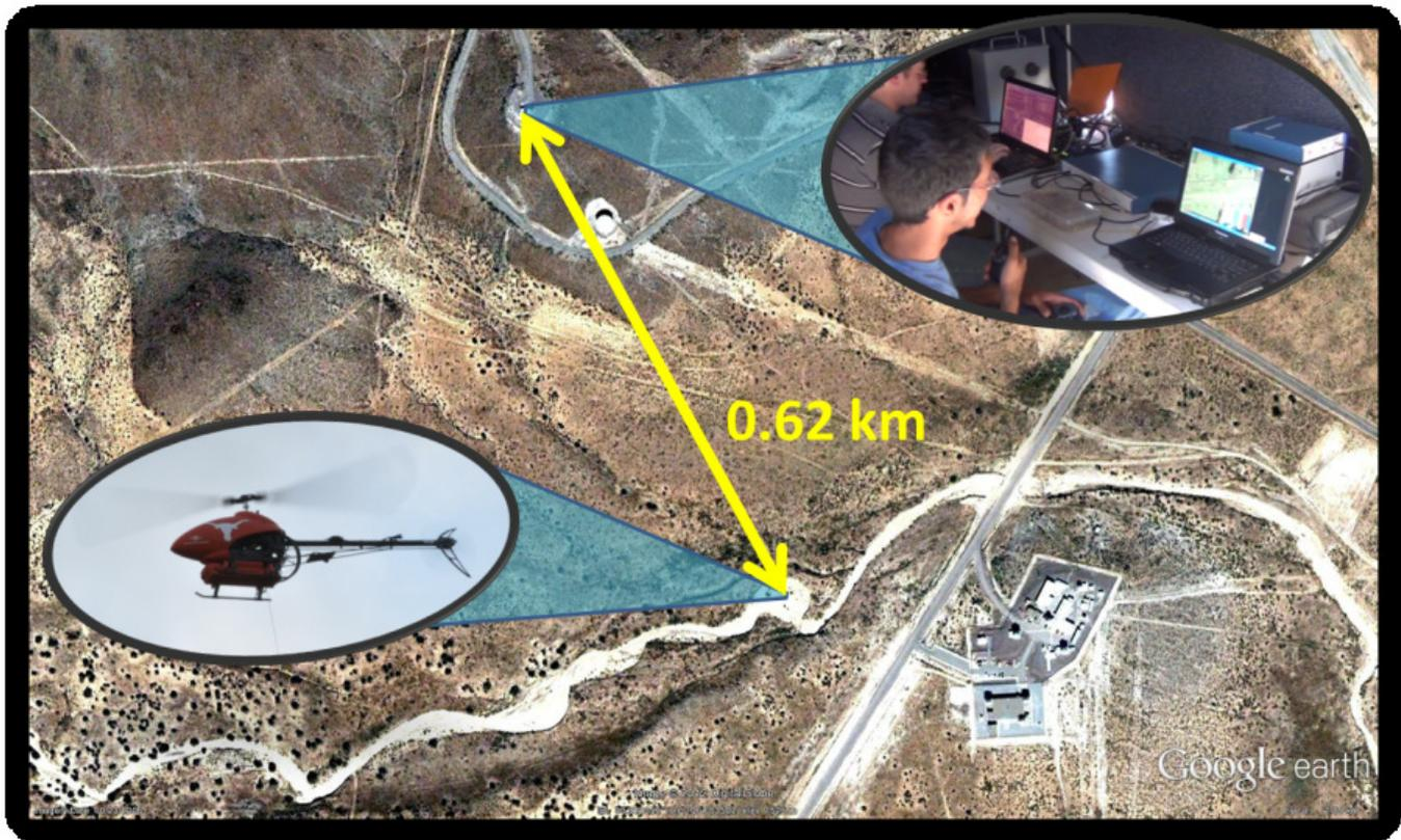
Fig. 6. Aerial view of the test site showing the spoofer location on a hilltop and the UAV site approximately 0.62 kilometers away.
