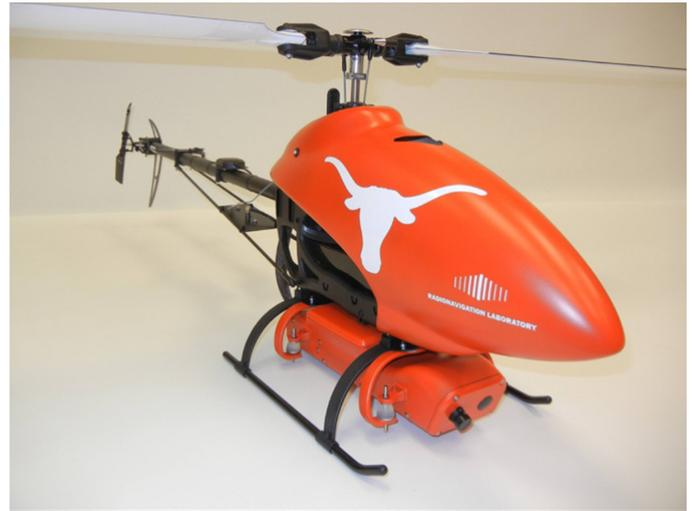
Fig. 4. The Hornet Mini unmanned aerial vehicle (UAV), owned by the UT, used in the spoofing tests.
