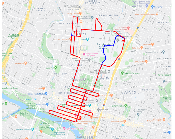
Fig. 7. Test route through The University of Texas west campus and Austin downtown. These areas are the most challenging for precise GNSS-based positioning and thus would benefit the most from radar-based positioning. The route was driven once on a weekday and again on the weekend to evaluate robustness of the radar map to changes in traffic and parking patterns. Red is the mapping run (May 12), blue is the localization run (May 9). A prior map is not available in the visible blue areas.
