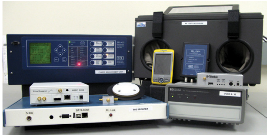
▲ SPOOFING TESTBED at the University of Texas Radionavigation Laboratory, an advanced and powerful suite for anti-spoofing research. On the right are several of the civil GPS receivers tested and the radio-frequency test enclosure, and on the left are the phasor measurement unit and the civil GPS spoofer.
