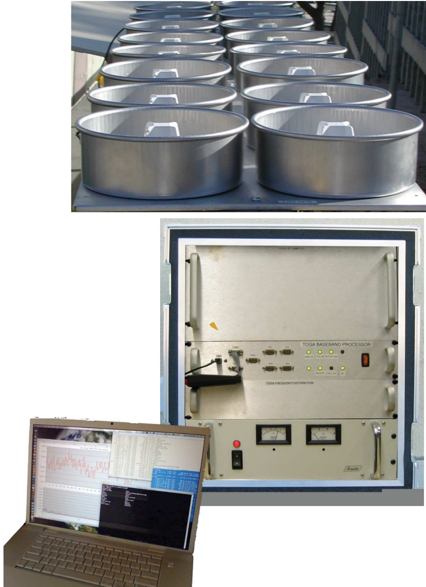
FIGURE 10. JPL's TOGA (Time-shifted, Orthometric, GNSS Array) instrument.
