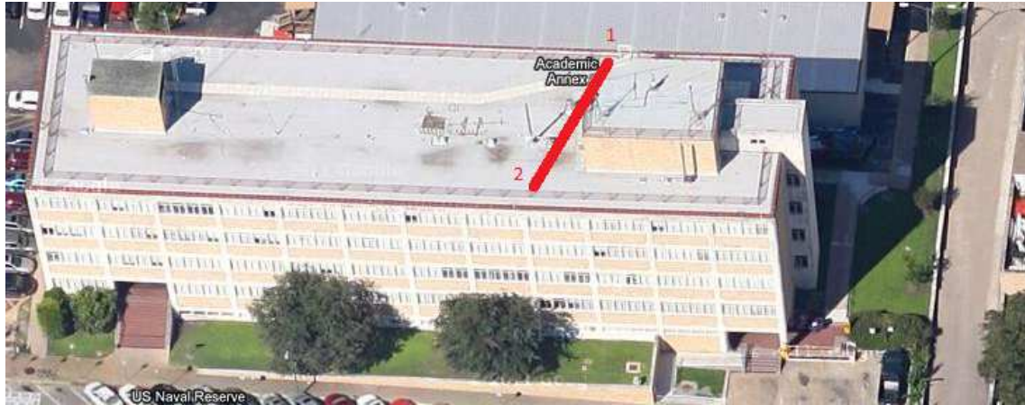
Figure 6.1: Picture showing the approximate locations of the two antennas used for the static test. Antenna 1 is the reference antenna, which is also used as the reference antenna for the dynamic test.
