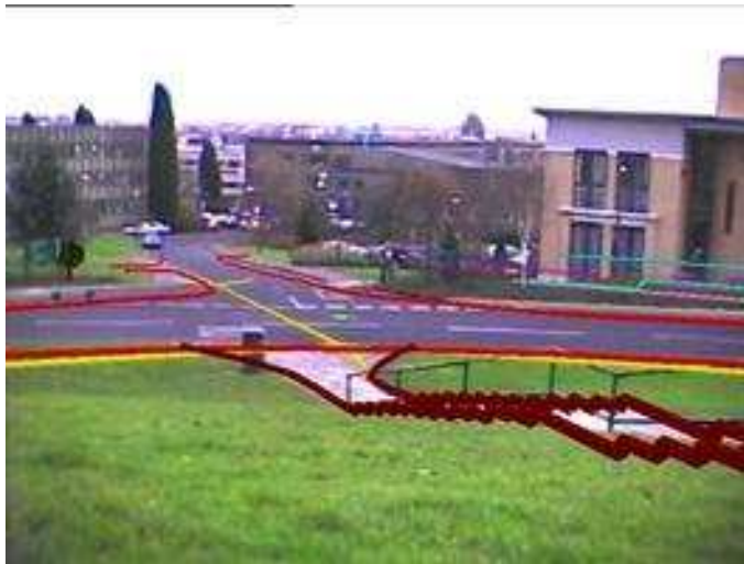
Figure 1.4: An image produced by an AR system developed by researchers at the University of Nottingham showing subsurface utilities overlaid onto the real world image in the background [4].
