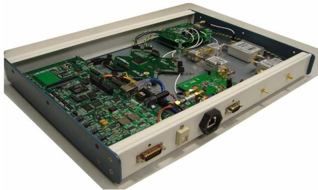
Fig. 9. The Cornell GRID receiver – the hardware platform for the receiver-spoofers.
