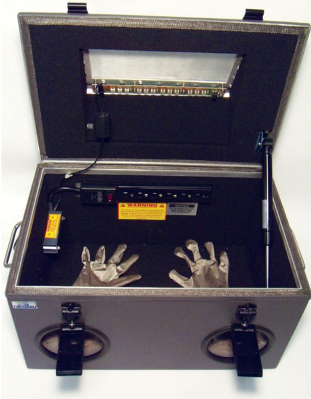
▲ **FIGURE 2** RF-shielded test enclosure. Jammers were operated inside the enclosure to prevent emission of their RF signals.
