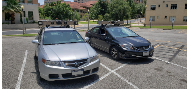
Fig. 1: The University of Texas Sensorium is a platform for automated and connected vehicle perception research. It includes stereo visible light cameras, an industrial grade IMU, one to three automotive radar units, a dual-antenna, dual-frequency software-defined GNSS receiver, 4G cellular connectivity, and a powerful internal computer.
