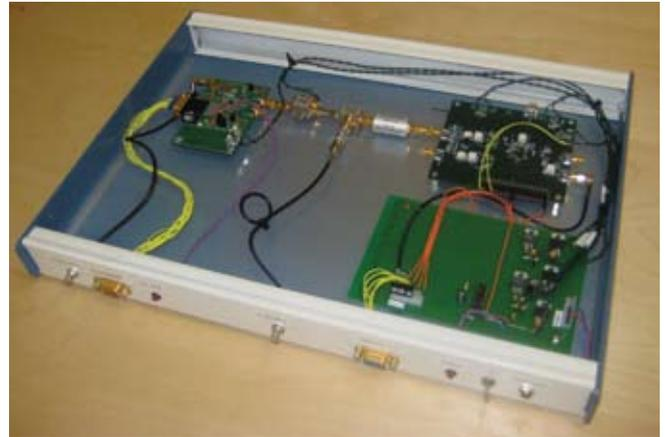
Cornell University GRID software-defined GPS receiver (left) RF transmitter prototype hardware (right)
