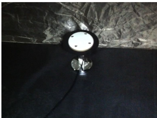
Fig. 5. Picture of the receive antenna inside the RF shielded tent which was pulling in both the authentic and spoofed signals to feed to the victim receiver.
