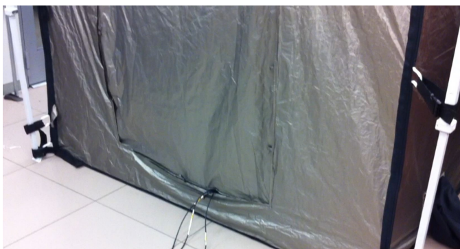
Fig. 3. Picture of the outside of the RF shielded tent with cables for the antennas.
