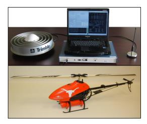
Figure 11: Spoofer hardware and target RUAV.
