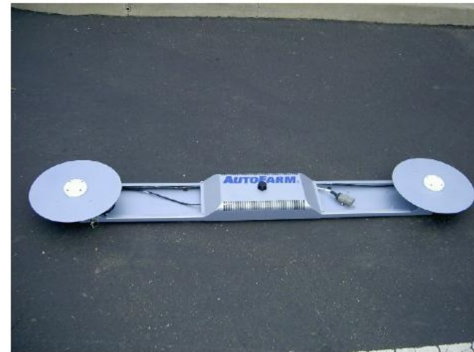
AutoFarm roof array with 146 cm baseline
