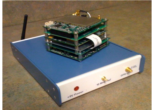
Fig 7. Two different form factors are available for the CASES receiver. The smaller one (top) is designed to fit inside a Cubesat.
