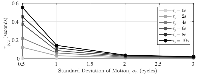
Fig. 4. Results of a Monte-Carlo-type simulation study showing the phase error correlation time \tau_{\phi,u} as a function of the standard deviation and correlation time of the antenna dynamics, \sigma_p and \tau_p , respectively. It is clear that \tau_{\phi,u} decreases exponentially in \sigma_p and is approximately linear in \tau_p .
