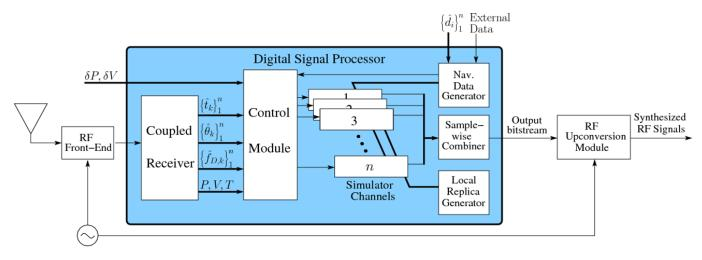
Fig. 2. A block diagram of the Spoofer.
