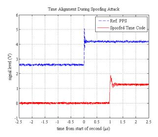
Fig. 14. Time alignment of the reference PPS (top blue dashed line) and the spoofed IRIG-B time code (bottom red line) at the end of the spoofing attack.
