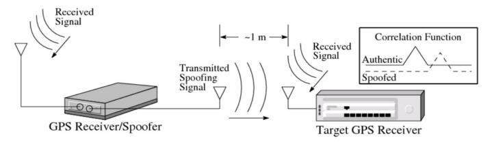
Fig. 3. A diagram of a proximity spoofing attack.
