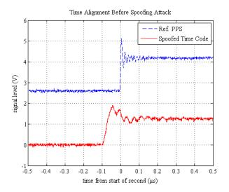
Fig. 13. Time alignment of the reference PPS (top blue dashed line) and the spoofed IRIG-B time code (bottom red line) before the spoofing attack began.
