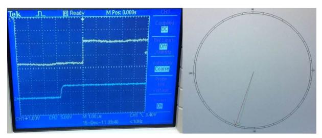
Fig. 9. Pictures of the oscilloscope (left) and synchrophasor (right) screen at about 620 seconds into the test, which is marked as point 2 in Fig. 7.
