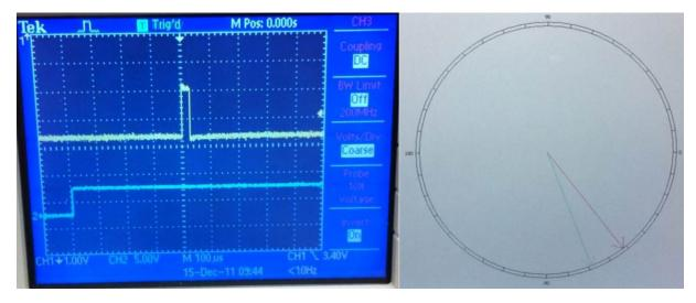
Fig. 11. Pictures of the oscilloscope (left) and synchrophasor (right) screen at about 870 seconds into the test, which is marked as point 4 in Fig. 7.
