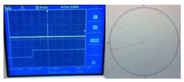
Fig. 12. Pictures of the oscilloscope (left) and synchrophasor (right) screen at about 1370 seconds into the test, which is marked as point 5 in Fig. 7.
