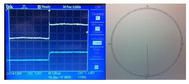
Fig. 8. Pictures of the oscilloscope (left) and synchrophasor (right) screen at the start of the test, which is marked as point 1 in Fig. 7.
