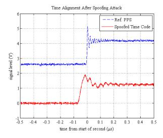
Fig. 15. Time alignment of the reference PPS (top blue dashed line) and the spoofed IRIG-B time code (bottom red line) after the spoofing attack ended.
