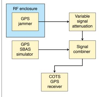
▲ FIGURE 6 Block diagram of the test procedure and equipment used to determine the GPS jammers' effective ranges.
