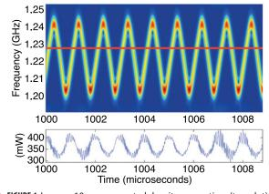
▲ FIGURE 4 Jammer 10 power spectral density versus time (top plot), with resolution of about 3 MHz and color indicating relative power, and power versus time (bottom plot) in a 62.5-MHz band centered at the L2 carrier frequency.
