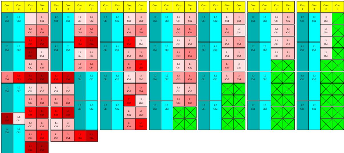
Fig. 6. Expected load balancing results with heterogeneous signal types, from well-balanced cases (toward left) to poorly-balanced cases (toward right) as a reduction in total channel load leaves a prominent L2C critical task. Each shade of red (blue) corresponds to a different L1 C/A (L2C) channel. Vacant processing blocks are colored green.
