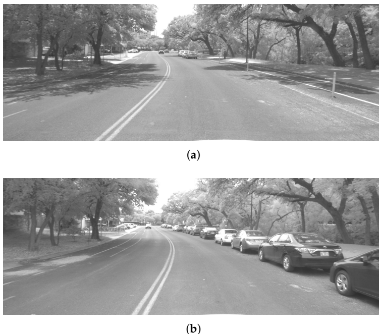
Figure 12. Different visual conditions on two days of data collection. (a) An image captured on the first day of data collection. Note the sharp shadows and absence of parked cars. (b) An image captured on the second day of data collection. Note the absence of sharp shadows and complete blockage of curb due to parked cars.
