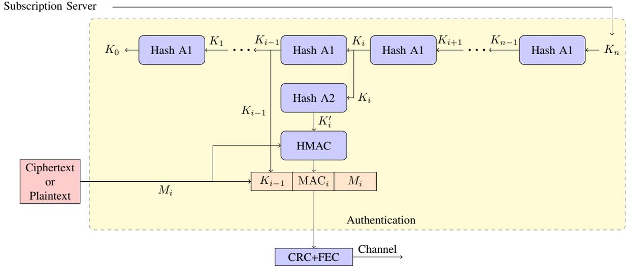
Fig. 3: Authentication processes at the TRNS pseudolite, which include one-way key chain generation, MAC generation, and broadcast packet formation.
