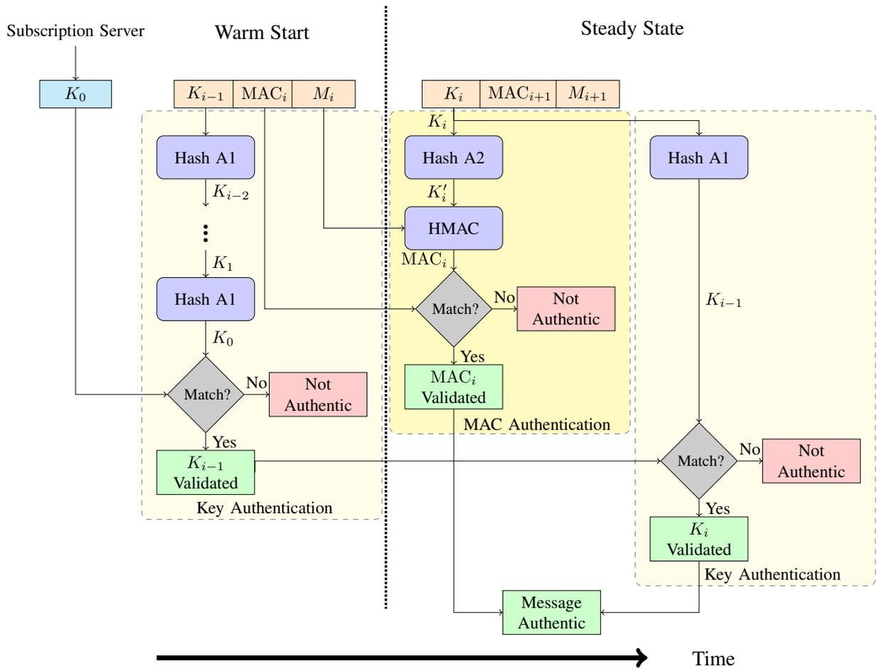
Fig. 4: Authentication processes within the TRNS receiver, which includes key validation during bootstrapping, and both key and MAC validation during steady-state phase.
