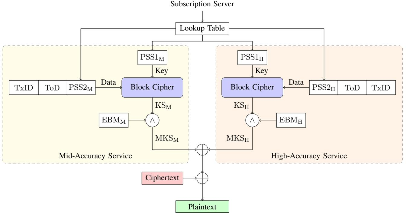
Fig. 2: Proposed TRNS NME scheme from the perspective of a high-accuracy service receiver. Note that in the high-accuracy receiver, both mid- and high-accuracy key streams are computed in order to decrypt the entire message.
