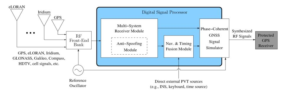
The GPS Assimilator modernizes and makes existing GPS equipment resistant to jamming and spoofing without requiring hardware or software changes to the equipment
