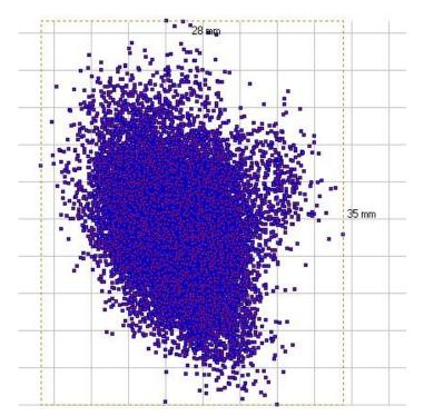
Horizontal scatter plot of final PDGPS adjustment at highest temporal resolution with bounding box (upward: north; right: eastward).
