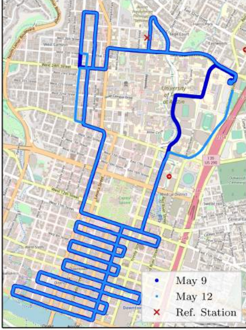
Fig. 7: Overview of the CDGNSS reference station position and routes driven through the urban core of Austin, Texas in the TEX-CUP urban positioning datasets. Routes differ slightly from May 9 to May 12 due to road closures.
