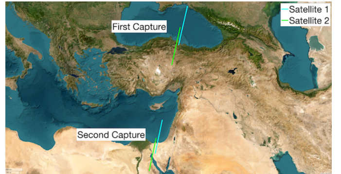
Fig. 4: Ground tracks of a pair of LEO-based receivers during the two 60-second captures over the Eastern Mediterranean. Both satellites are moving from north to south.
