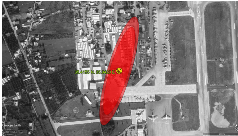
Fig. 8: Estimated transmitter location overlaid on 95 and 99% horizontal error ellipses. The location is coincident with an airbase on the coast of Syria.
